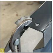
Warning: be careful not to damage the plate chalking. Place tape or another type of material between the clamp and the plate.
